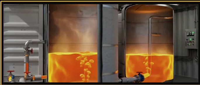
03 The insulated chambers keep the high temp of the liquid 24/7.
